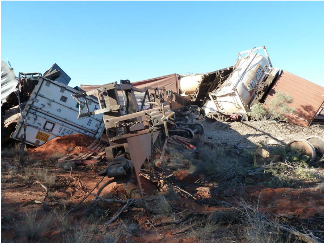
Figure 2: Derailed wagon and wreckage about 100m from the point of derailment
